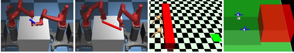
Figure 2: Screenshots of two of our manipulation tasks and our locomotion tasks. From left to right: corkscrew rotating, bar pickup, ant push, soccer. These tasks are all designed to require two agents. We learn policies for these tasks given only sparse binary rewards, by encouraging synergistic behavior via intrinsic motivation.
